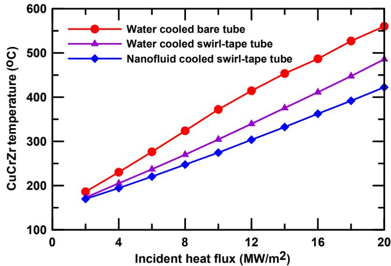
Fig. 3. Maximum CuCrZr temperature.
