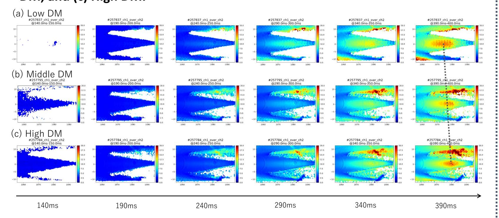
• The lower DM indicates that the recombination region is upstream and larger, while the higher DM corresponding to high- $T_i$  shows that the MAR region is pushed downstream.
