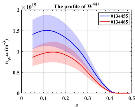
Figure 2 Comparison of  $W^{44+}$  density profile by VUV spectrometer during B powder injection for two shots with the same plasma parameters. The cumulative conditioning effect of B powder injection on W was suggested as B powder was successively injected between the two shots.
