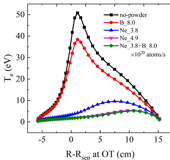
Figure 3 SOLPS-ITER simulated outer target electron temperature profiles for interesting cases labelled as the figure legend
