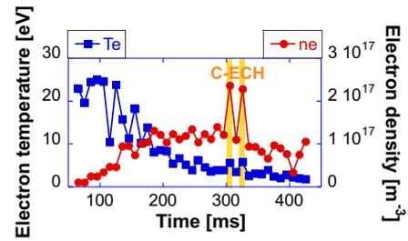
FIG. 3. Time evolutions of electron temperature (blue line) and electron density (red line) at ESP#3.
