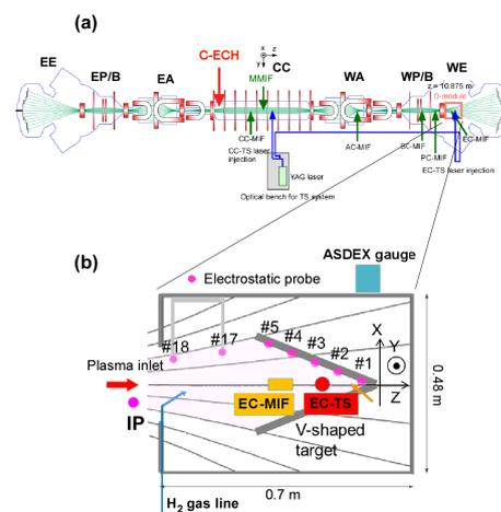
FIG. 1. Schematics of the experimental setup of GAMMA 10/PDX (a), and the divertor simulation experimental module (b).
