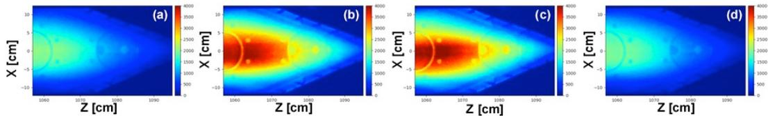
FIG. 5. H $\alpha$  images at  $t = 300.4 \text{ ms}$  (a),  $301.2 \text{ ms}$  (b),  $310.0 \text{ ms}$  (c), and  $310.8 \text{ ms}$  measured by HSCAM.
