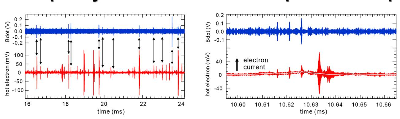
(a) Magnetic field fluctuations measured by the B-dot probe (top, blue) and electron current (bottom, red) at the plasma periphery measured by a high-energy electron probe. (b) Enlarged view of the fluctuation signal detected by the highenergy electron probe (bottom, red), along with its numerically low-pass filtered waveform (light blue), in comparison with the B-dot probe signal (top, blue).
