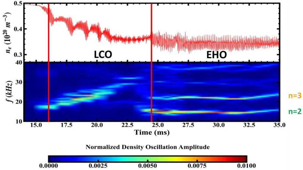
Fig. 2. Density oscillation signal at normalized poloidal flux of 0.95 outer mid-plane during 15~35 ms and its spectrogram. The temporal resolution of the signal is  $6.48 \times 10^{-6}$  s. The peaked oscillation with frequencies of 15 and 22.5 kHz in the EHO phase come from  $n=2$  mode and  $n=3$  mode, respectively.
