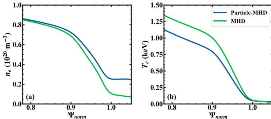
Fig. 1. (a) The toroidal averaged electron density and (b) electron temperature profiles at outer mid-plane in the coupled particle-MHD (blue) and pure MHD (green) simulations.
