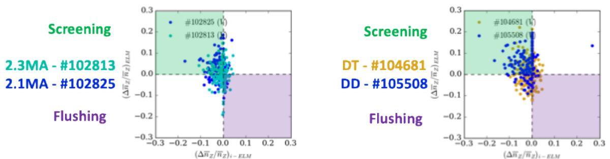
1: Screening vs flushing analysis of bolometer data for 2.1MA (blue) and 2.3MA (green) plasma (left figure) and for a DD plasma (blue) and a DT plasma (gold) plasma (right panel). Screening and flushing regions of plots indicated by colour.
