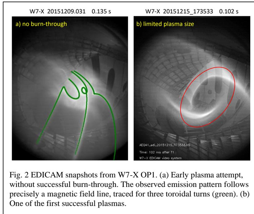
Fig. 2 EDICAM snapshots from W7-X OP1. (a) Early plasma attempt, without successful burn-through. The observed emission pattern follows precisely a magnetic field line, traced for three toroidal turns (green). (b) One of the first successful plasmas.
