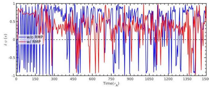
Figure 4. Time evolution of the phase difference between the density and electric potential fluctuations for the  $n=16$  mode. The blue lines represent results without RMP, while the red lines represent results with RMP.
