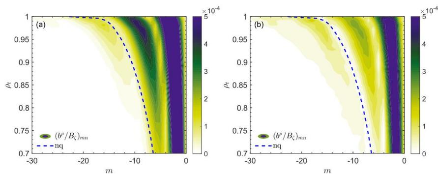
Figure 1. The calculated (a) vacuum field, (b) plasma response field using CLTx code.
