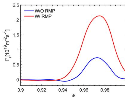
Figure 2. Simulated radial particle fluxes averaged over magnetic surfaces for the cases with (red) and without (blue) perturbed fields induced by RMP.
