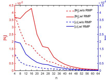
Figure 3. The amplitudes of density and potential fluctuations for different toroidal mode numbers. The red line represents the density perturbation amplitude, the blue line represents the electric potential perturbation amplitude. Solid lines indicating results with RMP and dashed lines indicating results without RMP.
