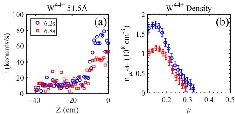
Figure 2. (a) chord-integrated line intensity and (b) density distribution of  $W^{44+}$  measured by EUV.
