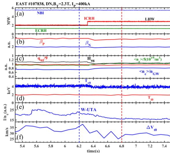
Figure 1. The time traces of (a) heating power, (b) plasma beta, (c) line-averaged density, Greenwald density fraction,  $q_{95}$  and  $H_{98}$ , (d) central electron and ion temperature, (e) intensity of W-UTA line normalized to electron density (f) central relative toroidal rotation velocity of EAST discharge #107838.
