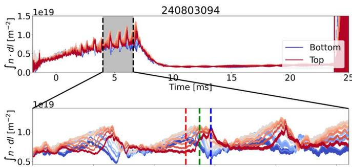
**Figure 1:** Measurements from an NBI shine-through diagnostic provide time resolved, line-integrated density measurements across the plasma. These agree very well with single-chord interferometry measurements and provide more information about the spatial fluctuations. In this particular shot, a gate valve magnetized by the high field was partially closed, leading to an unexpected oscillatory behavior.
