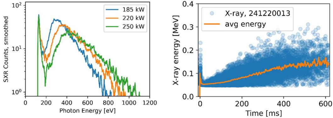
**Figure 2:** Left: increased ECH power is reflected in the measured soft X-ray spectrum. Right: Hard X-ray measurements from a high power, low density ECH shot show signal long after the 20 ms of input power. In the afterglow, cold electrons scatter and deconfine more quickly, leading to 'evaporative heating'.
