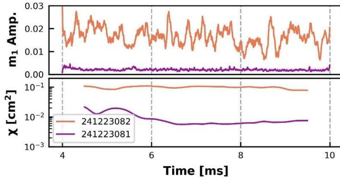
**Figure 1:** Top, amplitude of  $m=1$  plasma oscillations, as measured by a 20 chord AXUV diode array. Bottom, the y-axis parameter represents the phase space area of fluctuations in the centroid position and radius of the emission profile. The factor of 10x reduction in fluctuations is due to end-ring biasing applied in shot 241223081 and absent in 241223082.
