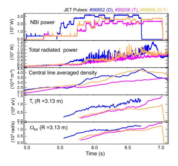
Best performance ITB pulses are at different NBI powers in D, T, D-T:
