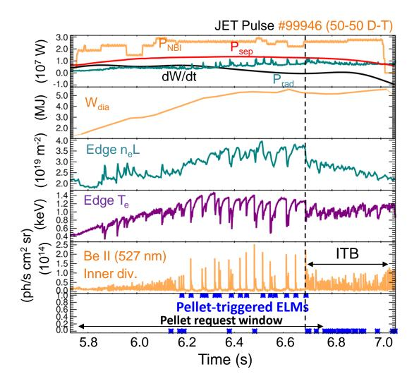
HFS pellet pacing to mitigate type I ELMs for W control (2mm, 45 Hz, D pellets)
