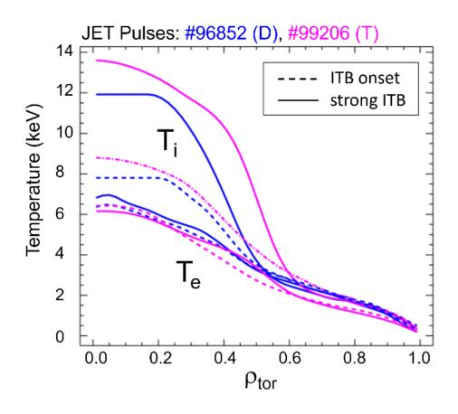
Ion ITB foot at larger radius in T than in D at fully developed ITB
