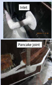
Targets of insulation reinforcement on an EF coil and examples of the reinforced parts
