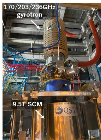
Fig. 1 The multi-frequency gyrotron (170/203/236 GHz) and SCM (up to 9.5 T) newly installed into QST's gyrotron test stand.
