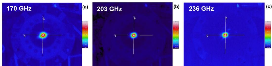
Fig. 2 Measurement of beam patterns at the output window at a) 170, b) 203, and c) 236 GHz.
