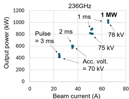
Fig. 3 Characteristics of output power versus beam current measured in short pulse operations at 236 GHz for 1 to 3 ms.
