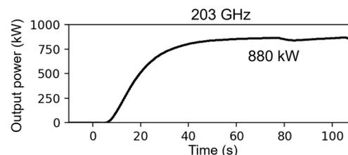
Fig. 4 The output power, measured with a dummy load, achieved to 880 kW in the 100s-operation at 203 GHz. The slow increase in power is due to the calorimetry.
