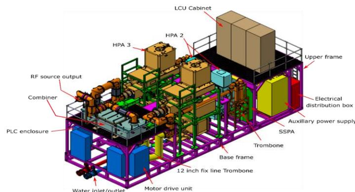
Figure 1: 3D view of RF source layout
