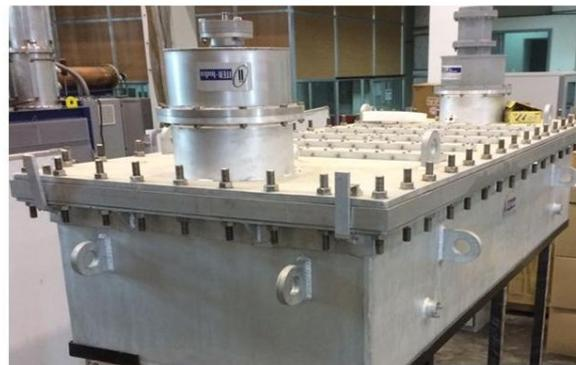
Figure 2 (a) VSWR response of the combiner (b) fabricated prototype combiner
