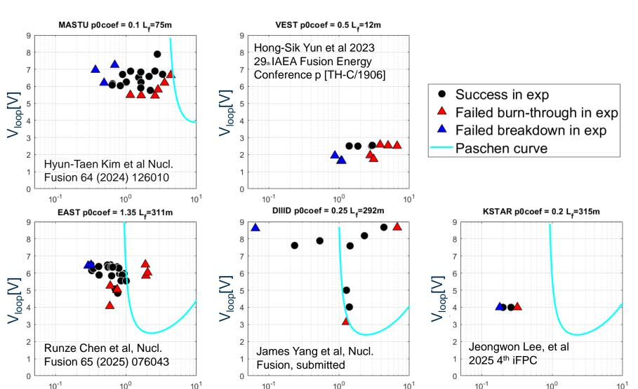
Failed burn-through at high  $p_0$ Failed burn-through at low  $V_{loop}$ Failed breakdown at low  $p_0$  $\rightarrow$ The hypothesis is valid for all devices.
