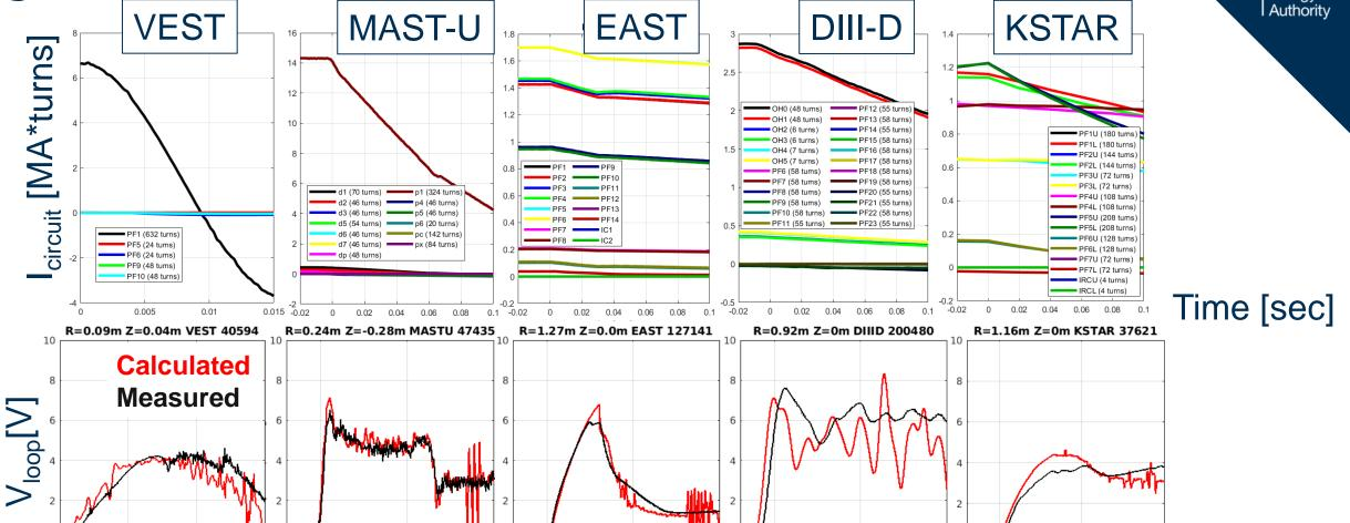
Calculated the measured V<sub>loop</sub> at the inboard mid-plane using the coil current time traces.
