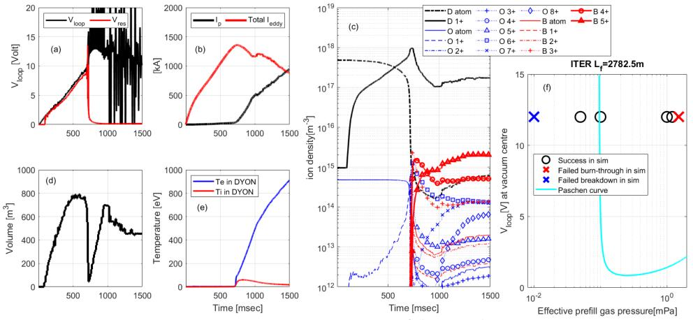
Machine description and coil current time traces are from IMAS (#105052). DYON predicts with 0.1% initial oxygen + physical sputtering of Boron
