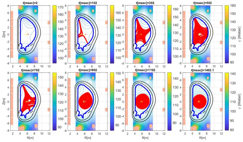
Machine description and coil current time traces are from IMAS (#105052). DYON predicts with 0.1% initial oxygen + physical sputtering of Boron
