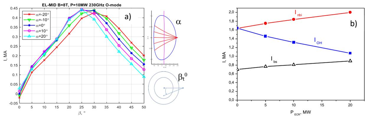
Fig. 2. a) Value of ECRF wave driven current at  $P_{ECRH}=10$  MW,  $B_t = 8$ T, 230 GHz, depending upon injection angles ( $\alpha$  – with respect to equatorial plane,  $\beta_t^0$  – with respect to perpendicular direction in equatorial plane, b) plasma currents upon  $P_{ECRH}$  (fixed wide ECRF wave absorption profile at  $\rho=0.4$ ,  $P_{NBI}= 20$  MW)
