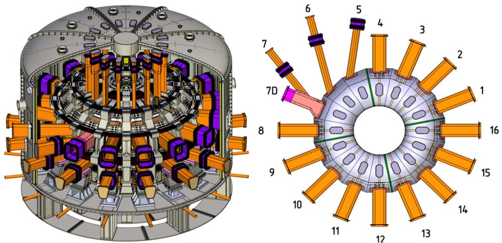
Fig. 1. TRT conceptual design with port numeration for diagnostic systems distribution
