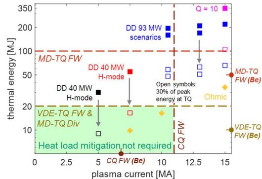
Fig. 3: Thermal energy limits for W first wall (FW) and planned scenarios during SRO and FPO.
