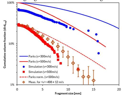
Fig. 2: Cumulative fragment volume (normalized to the original pellet volume) comparing Parks's model with simulations for two pellet impact velocities and with one laboratory shattering characterizations (averaged over five repetitions and (both scaled to the minimum detectable fragment size). Dashed line shows corresponding Parks's model scaled to measurements.
