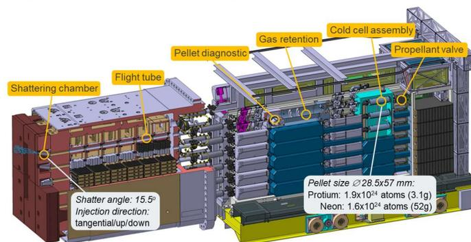
Figure 1: Shattered pellet injector components in one of the equatorial port cells.
