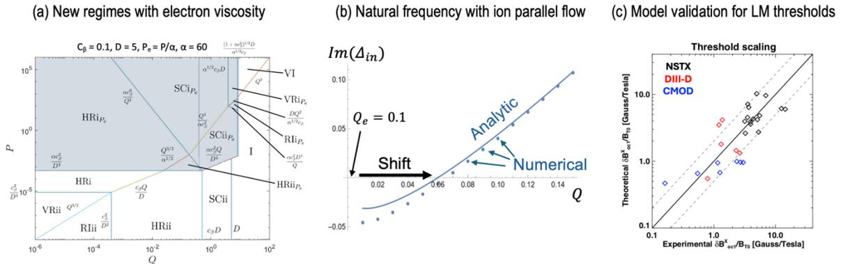
Fig. 1 (a) Newly identified regimes due to electron viscosity as a function of normalized viscosity ( $P$ ) and rotation ( $Q$ ) as colored in blue. (b) Shift of natural frequency  $Q$  for  $\Delta_{in} = 0$  from  $Q_e$  due to ion parallel flow in high  $\beta$  ( $c_\beta \rightarrow 1, D = 0, P = 0$ ), as verified by high-order matching theory and numerical modeling. (c) Comparison of locked mode thresholds between GPEC SLAYER modeling and experimental data.
