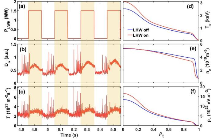
Figure 1. Plasma parameters of the ELM control experiment with LHW, including (a) LHW heating power, (b)  $D_\alpha$  emission intensity, and (c) particle flux measured by DLPs. Radial profiles of the fitted electron temperature (d), electron density (e), and electron pressure (f), with the horizontal axis  $\rho_t$  as the normalized toroidal flux.
