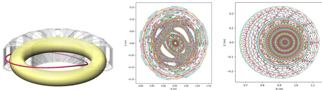
Fig 1. (a) Structure of helical coil in J-TEXT tokamak. (b) Poincaré plot of magnetic field topology in M3D-C1 simulation of J-TEXT disruption in presence of REMC. (c) Poincaré plot of M3D-C1 simulation with influence of RE current on MHD turned off.
