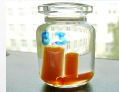
Cylinder blocks (in PE envelope) In acetone, D=4 и 7mm, L=11 и 17 mm
