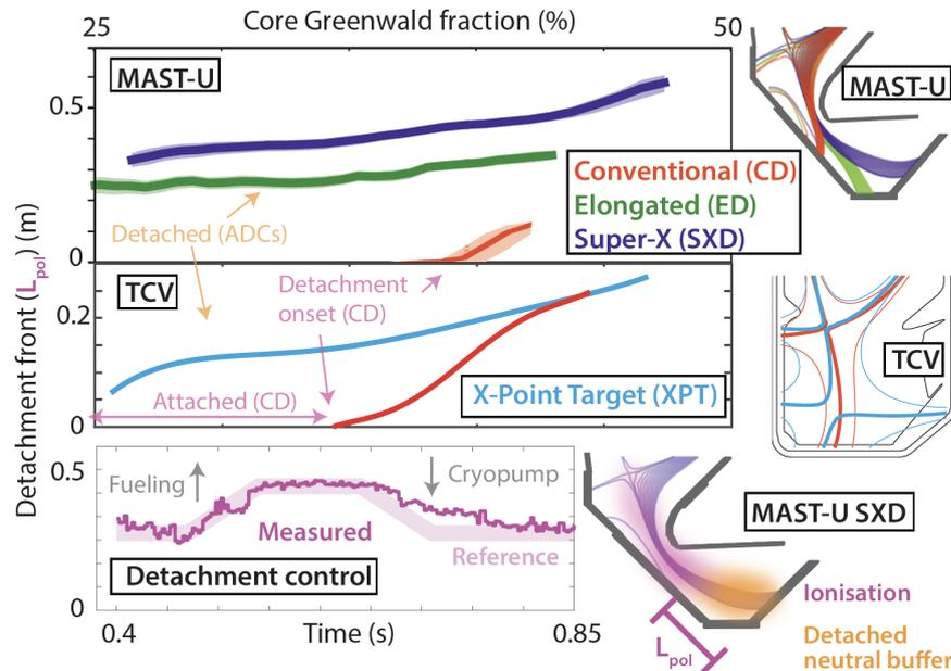
Figure 1: Detachment front evolution showing ADC benefits in terms of detachment access (front detached at lower core density) [3,5], sensitivity (reduced slope front movement) [3,5], operational window (larger window in which the front is between the target and X-point) [3,5] and detachment control [8].
