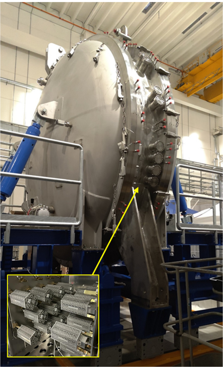
Completing SPIDER configuration: ongoing installation of new vessel module with NEG pumps and new RF solid-state amplifiers
