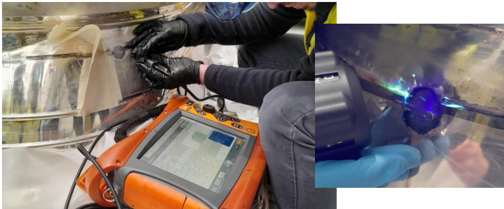
Systematic visual inspection & FPT
