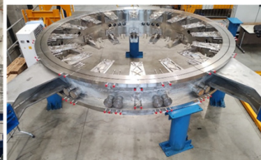
VEM at NBTf site, ready for NEG support panels installation
