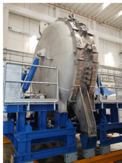
VEM at NBTf site, ready for NEG support panels installation
