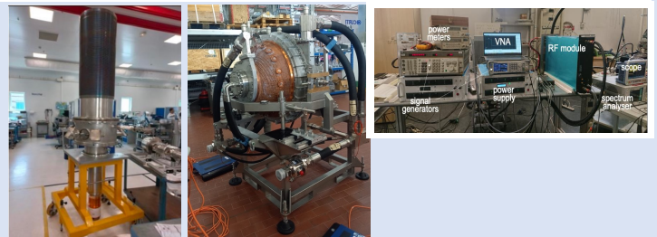
Left: pre-series gyrotron; middle: RF load; right: ICH solid state module.
