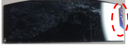
FIG. 11. The plasma-facing surface of a silicon sample. The location of a-C:H film deposition, which was in the shadow of the holder's fastening element, is shown by the dashed line.
