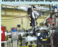
Fluorescence Profile Monitor (CIEMAT) Collect light from ionization of beam particles + residual gas
