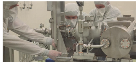
Fig. 3: Assembly work of the SRF beam line components in the clean room
