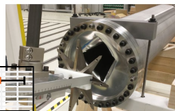
Li fire experiment demonstrating extinction with Ar gas
