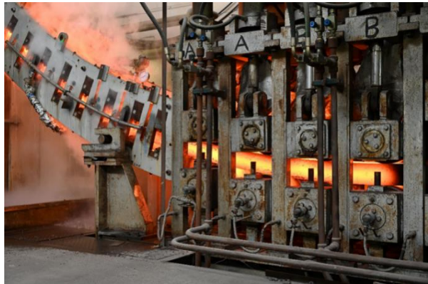
Figure 4: NEURONE project billet leaving the caster and entering the product straightener. Image Credit: Materials Processing Institute
