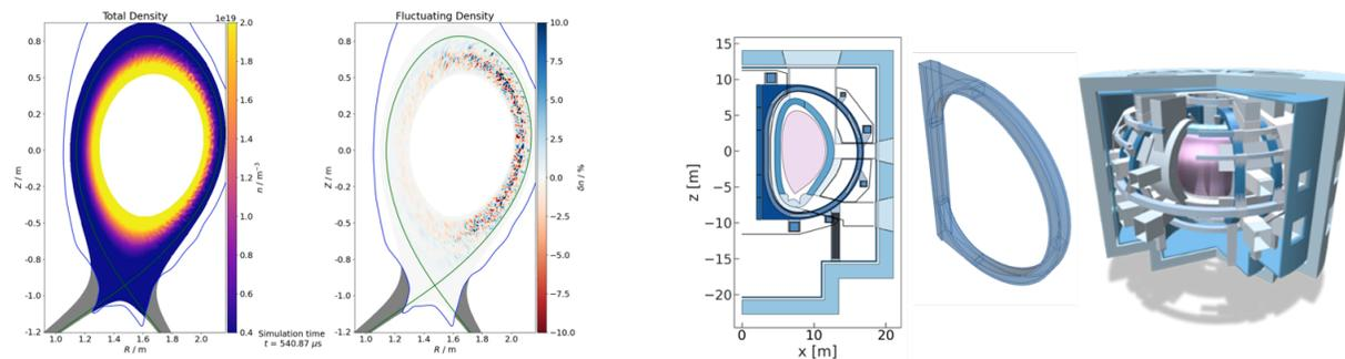
Fig. 1: Examples for important steps towards digital twins of partial or complete fusion systems: [Left] Turbulent transport in AUG, simulated with the fast full-f gyrokinetic GENE-X code. [Right] BLUEMIRA-generated CAD for DEMO: 2-D cross section, TF coil, and whole reactor 3D CAD.
