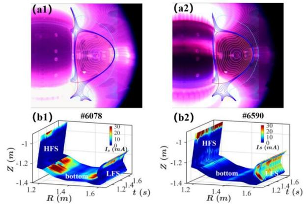
Fig.2 Comparative analysis of tripod and snowflake configurations. Fast camera image and configuration of the (a1) tripod and (a2) snowflake case, ion saturation current profiles by divertor Langmuir probes for the (b1) tripod and (b2) snowflake case.
