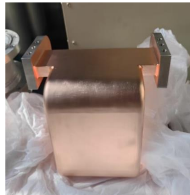
Antenna module 3D printing(56 pieces \phi 5\text{mm} TPMS cooling channels)
