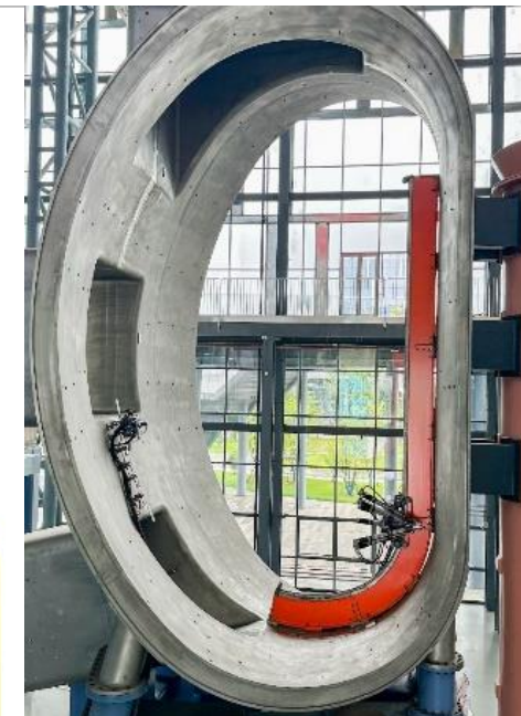
Online milling of field weld seam defects
