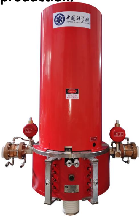
4.6GHz 500kW klystron with double output windows
