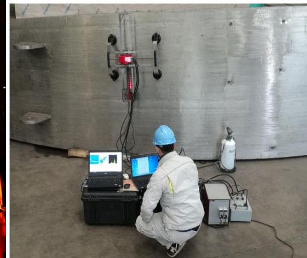
In-site automatic PAUT system
