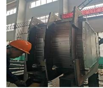
Full size welding mockup of straight leg and curve leg
