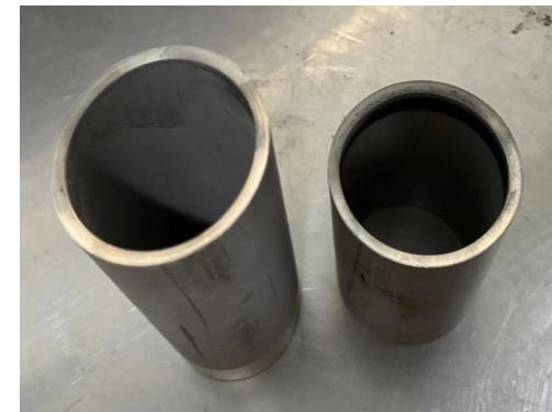
Debris-free cutting of 3 mm-thick 316L pipes(50, 60mm)
