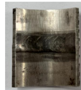
Achieved automatic TIG welding of 316L pipes without filler wire
