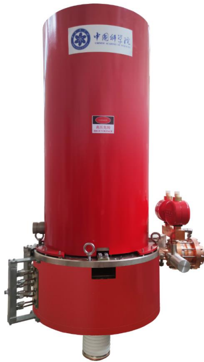
4.6GHz 500kW klystron with single output window
