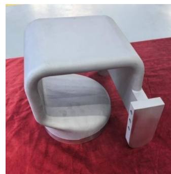
Antenna module 3D printing(56 pieces \phi 5\text{mm} TPMS cooling channels)
