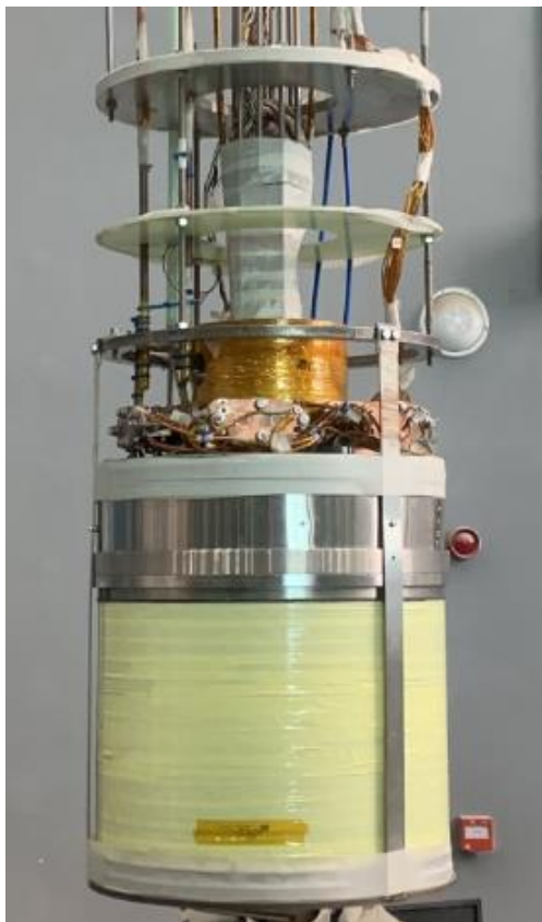
Self-Developed Background SC magnet (19T&70mm\ 15T&150mm)
