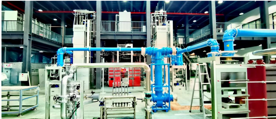
Fig.2 ICRF system. 3MW, 40-90MHz, CW. All components have been tested up to full power.
