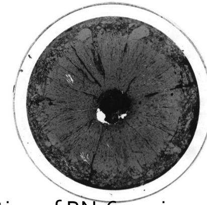
Cross-cutting of BN-600 pin
