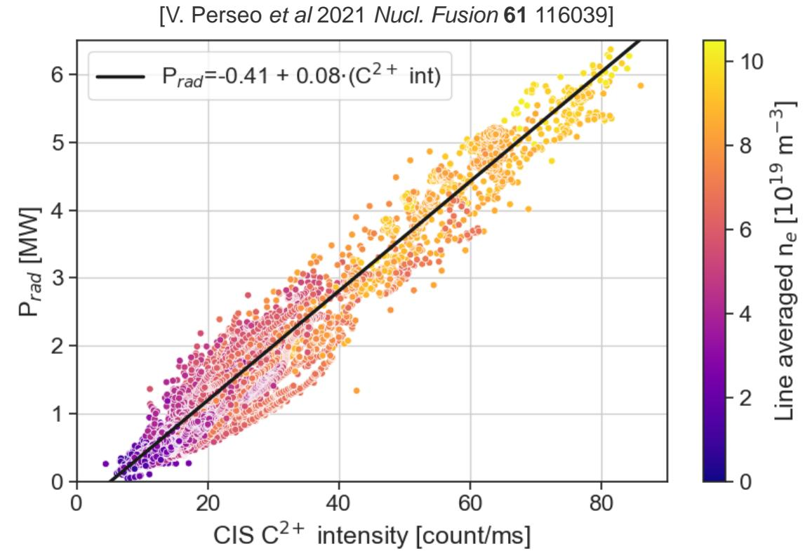
Plasma radiation proportional to  $C^{2+}$  intensity and plasma density → hydrogen fueling is our method to reach certain level of radiated power (and thus the SOL carbon concentration)
