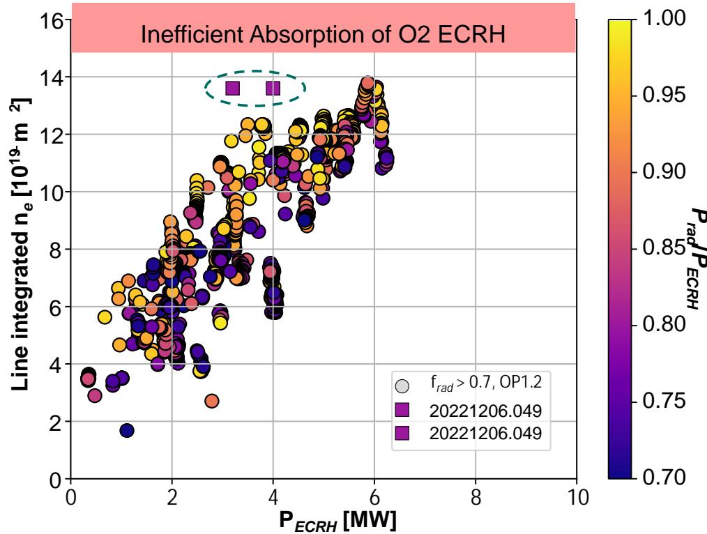
Scaling of the curve dependent on Zeff value → the smaller the impurity content (e.g. via boronisation or wall conditioning) the higher the necessary density
