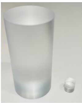
ITER pellet D = 28.5 mm L = 57 mm AUG pellet D = 8 mm L = 8 mm
