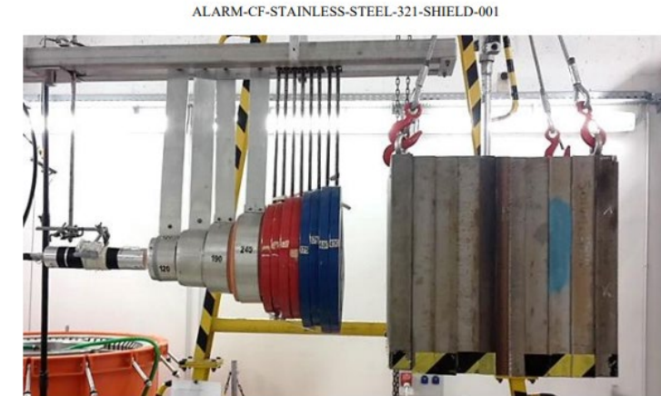
Figure 4. Photo of Stainless steel Block with Shielding Cone and Stilbene Detector.
