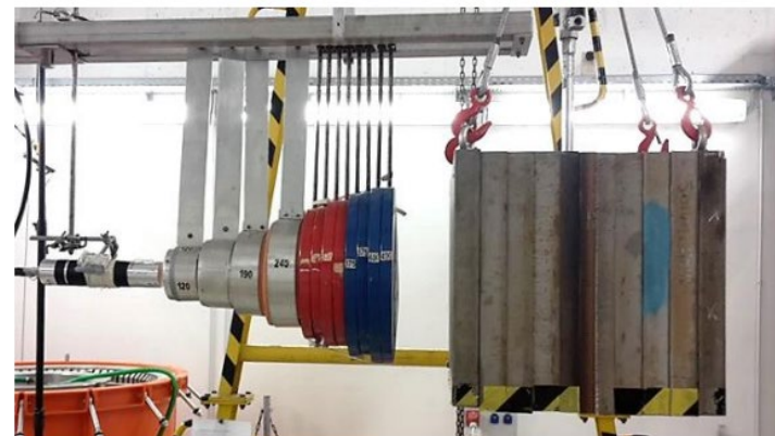
Figure 4. Photo of Stainless steel Block with Shielding Cone and Stilbene Detector.
