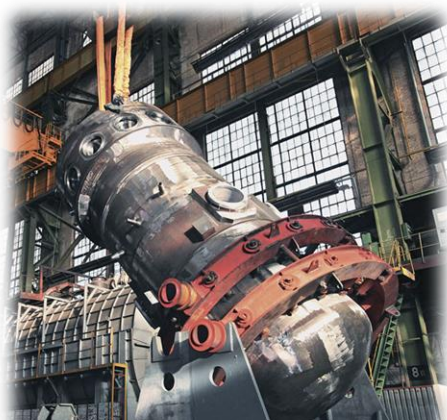
Reactor vessel installed in a special slipway
