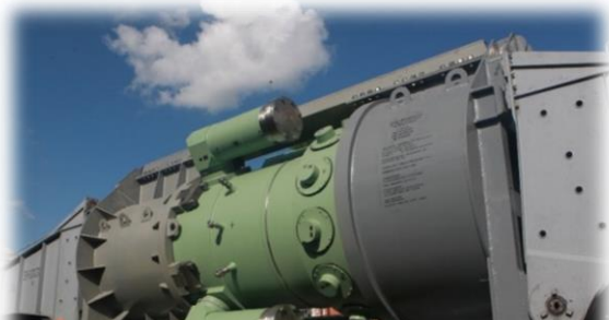
Transporting the RITM-200 steam generating unit
