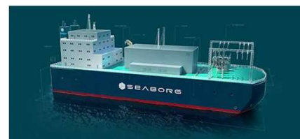
Figure 2. The Seaborg barge ship is one example of a marine application of Gen IV nuclear reactor technology. Photo from Seaborg Technologies.
