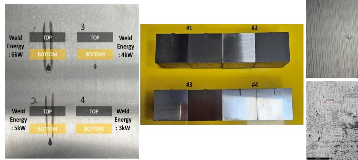
Chemical compositions and Pictures of 316L after laser welding and wire cut specimens for Vickers hardness and SE(EDAX point analysis) images
