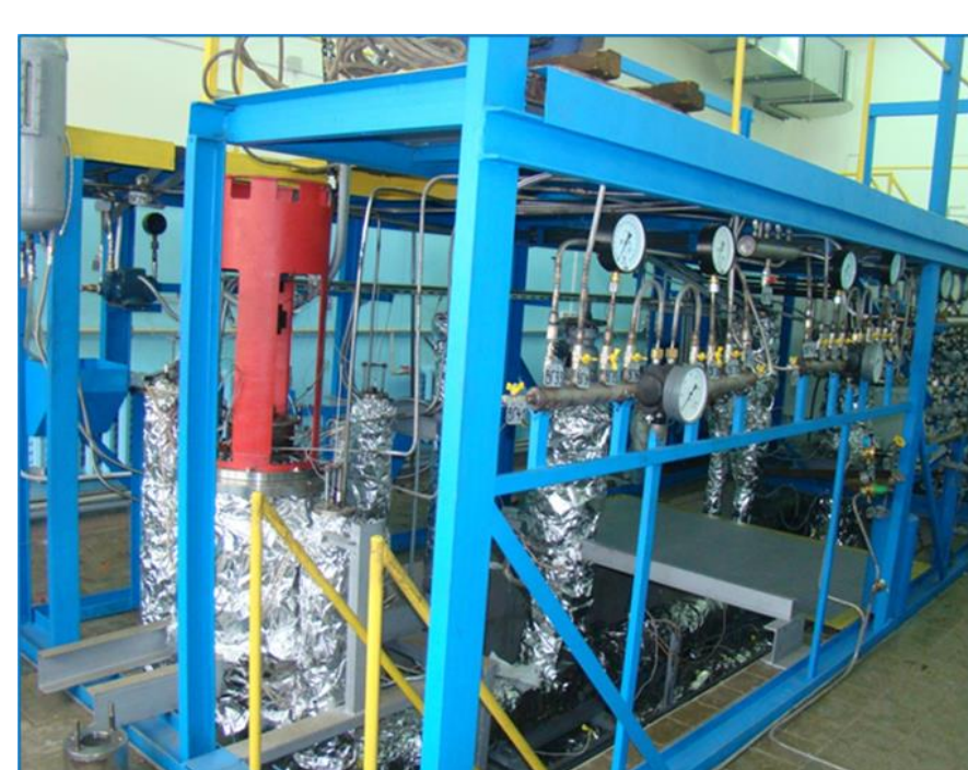
Test facility FT-4 and prototype of the axial-flow pump for liquid lead-coolant made in NNSTU
