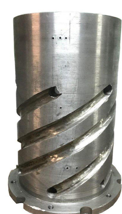
Test facility FT-4 and prototype of the axial-flow pump for liquid lead-coolant made in NNSTU
