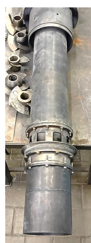
Test facility FT-4 and prototype of the axial-flow pump for liquid lead-coolant made in NNSTU
