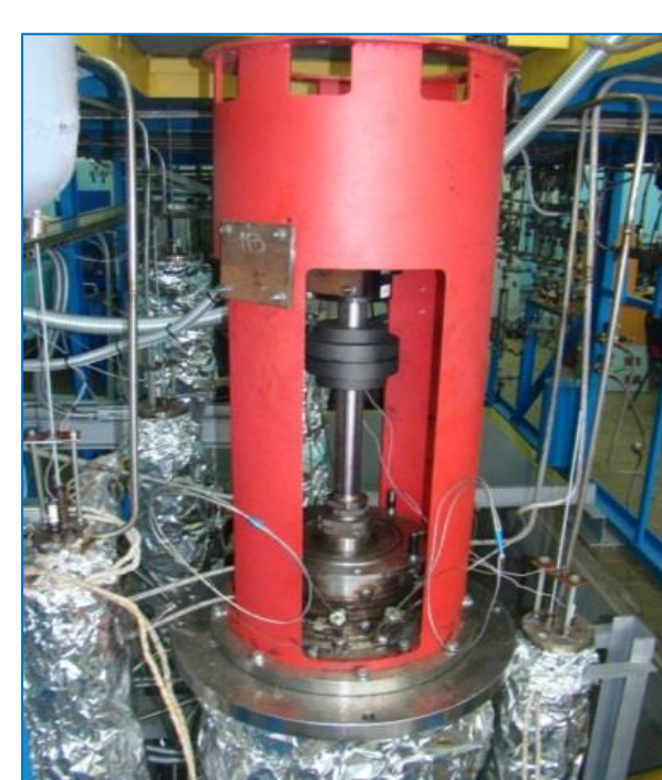
Test facility FT-4 and prototype of the axial-flow pump for liquid lead-coolant made in NNSTU
