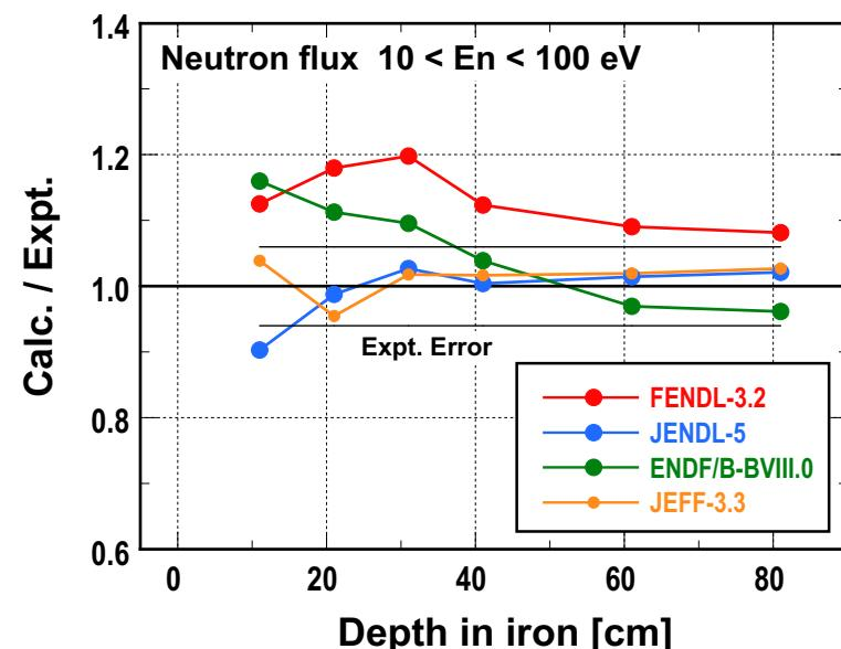
***FENDL-3.2b and ENDF/B-VIII.0 tend to overestimate measured neutron flux below 10 keV up to depth of 60cm!***
