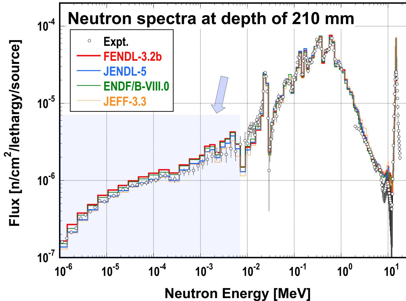
***FENDL-3.2b and ENDF/B-VIII.0 overestimate the measured neutron spectrum below 10 keV!***
