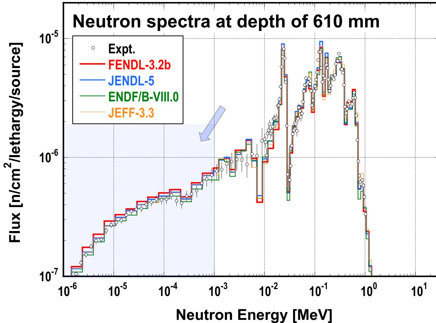
***FENDL-3.2b slightly overestimates the measured neutron spectrum below 1 keV !***
