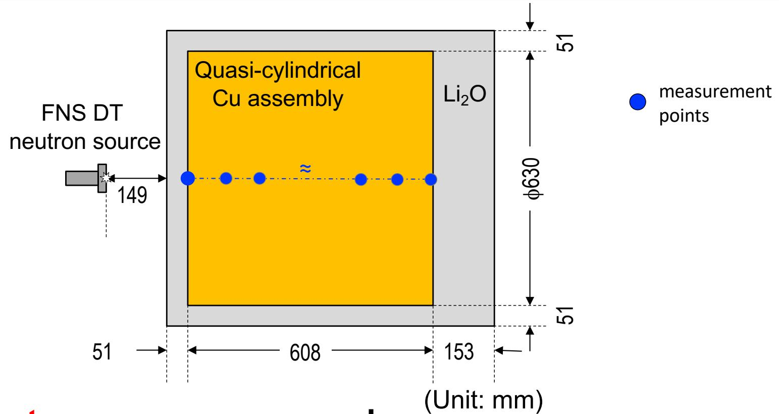
**Reaction rates were measured inside the copper assembly.**
