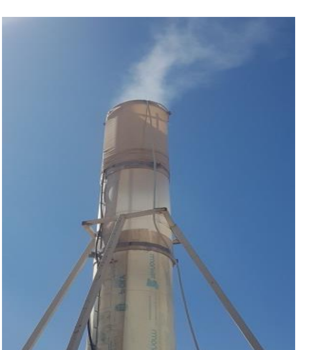
FIG. 9 Behavior of the fumes at the exit of the vortex tower chimney.
