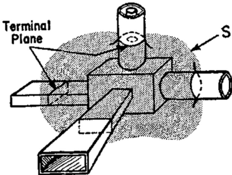
“A transmission line (waveguide) junction”
