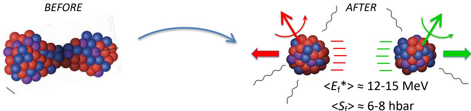
The (correlated) fragment spin distribution  $P(\mathbf{S}_L, \mathbf{S}_H)$  is sensitive to the fission mechanism
