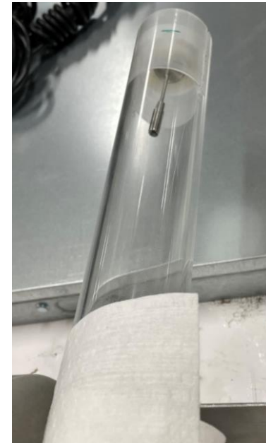
Target gas cell and target holder
