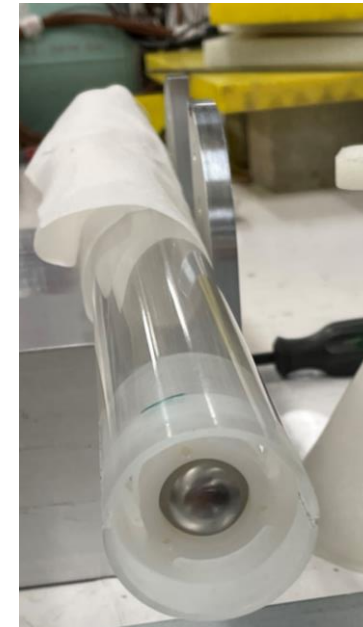
Target gas cell and target holder
