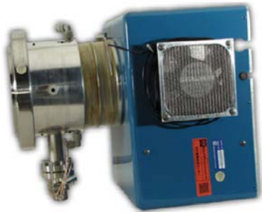
The Alphatross source is a compact, reliable source of light negative ions. A positive RF source injects immediately into a compact rubidium charge exchange cell.
